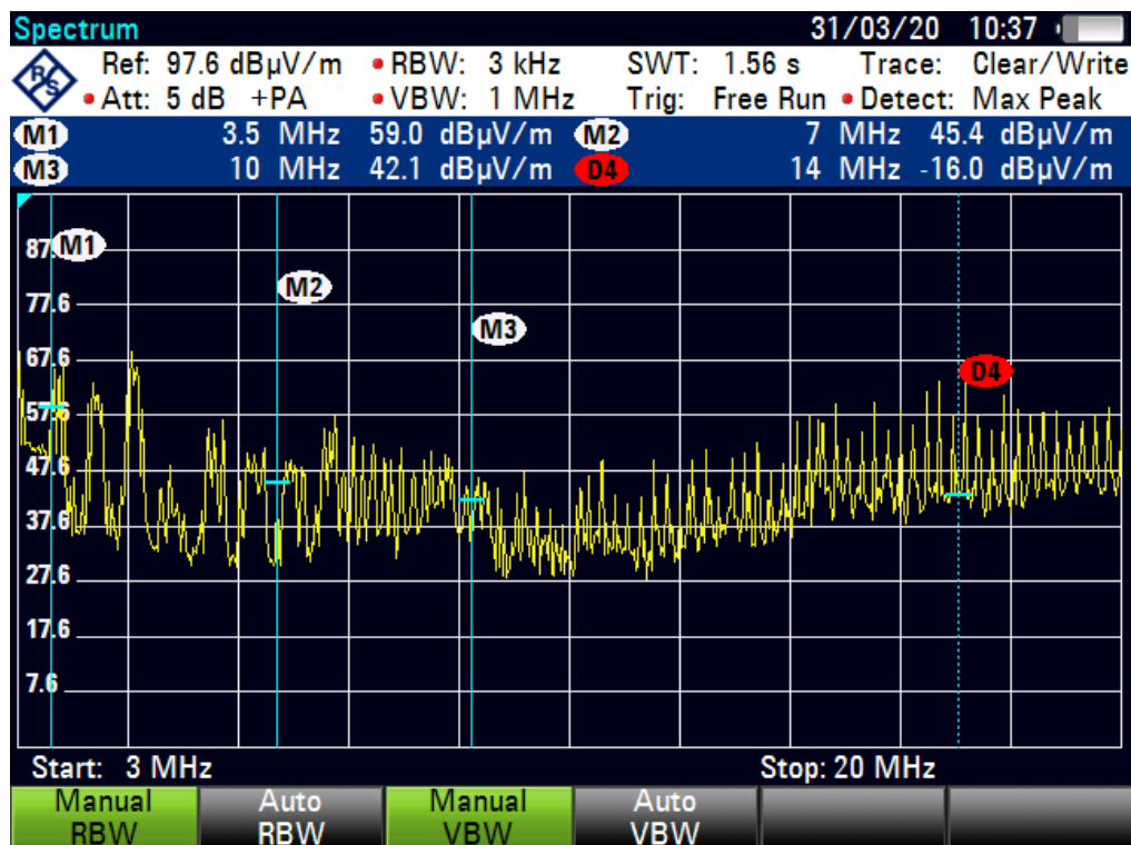
Figur 18: Utstrålad emission, vertikal polarisation.
