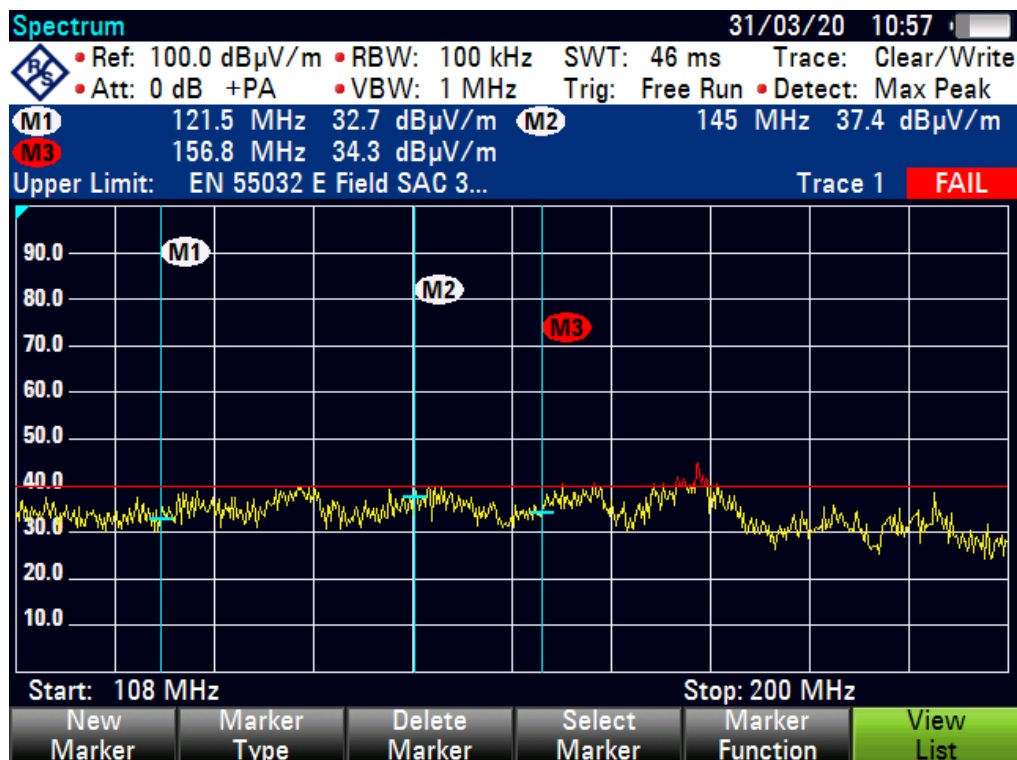
Figur 27: Utstrålad emission, vertikal polarisation.
