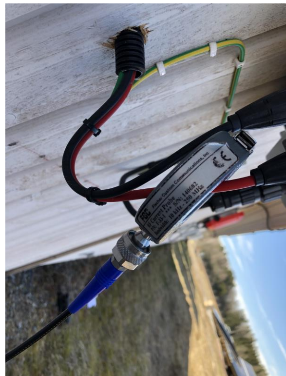
Figur 40: Fisher F-33-1 Strömprobe. s/n: 140682 kal: 2014-07-18
