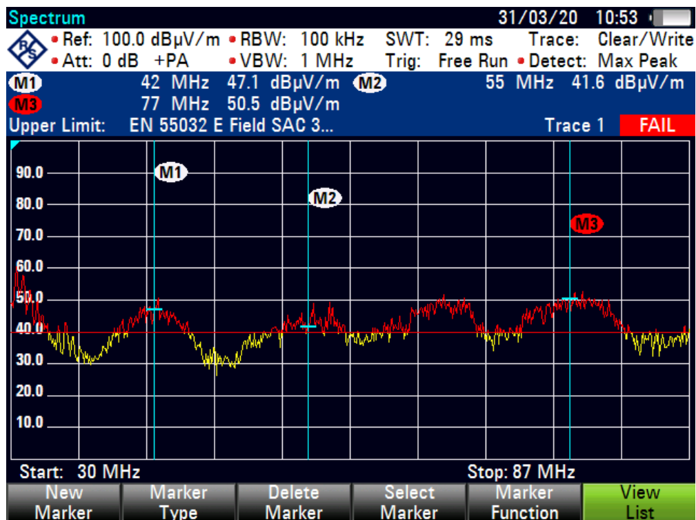
Figur 25: Utstrålad emission, vertikal polarisation.
