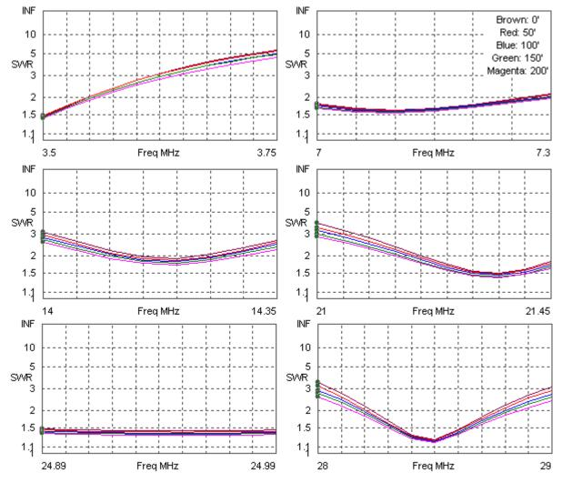
In-Band 50-Ohm SWR Sweeps: OCF Antenna and LMR500 Cable 50' above Average Ground Fig. 9
