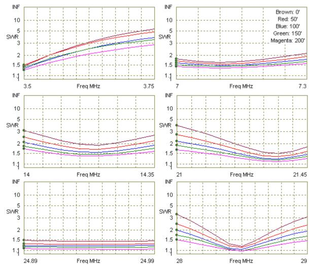
In-Band 50-Ohm SWR Sweeps: OCF Antenna and RG-58A Cable 50' above Average Ground Fig. 11
