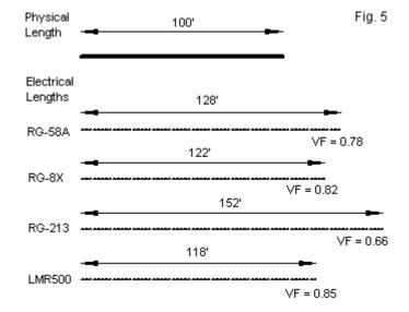
Transmission Line: Physical vs. Electrical Lengths
